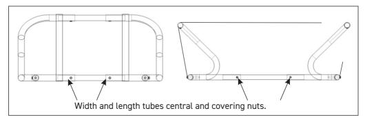
3.8 Once this is confirmed, screw the dome screws (E) into all twelve nuts and tighten securely with a 3mm allen key. The cradle can be fitted into the deck or rail.
