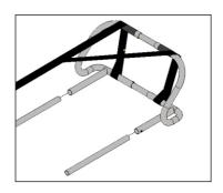
3.4 Slide the opposite arms without grip (A and D) into the other end of the length beams to join the cradle together. Ensure the length beams are evenly positioned between the arms before joining together.
