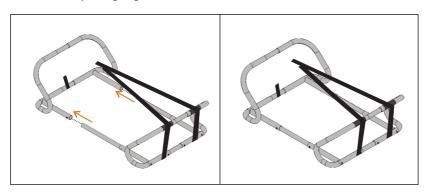
3.5 Position the liferaft in the cradle and slide the arms in or out accordingly to fit the desired liferaft.
