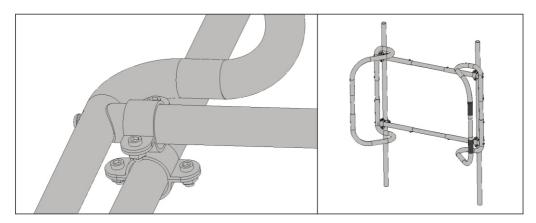
5.4 Once the cradle is secured to the vessel, **position the liferaft inside.** The arms can be rotated up and down to the lift the raft in and out. If this is not possible, the mounting brackets have been positioned in the wrong place and need re-positioning. Push the arms out when placing the raft inside. If vertically mounted, ensure the painter line of the liferaft is at the top. **Please continue to section 6.0 Strapping, P13.**
