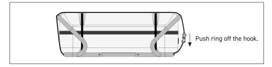
7.2 The side arms can be rotated up and down to lift the raft in and out. Push the arms out to remove the liferaft.
