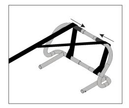
3.2 Repeat this process for the shortest strap (J) and left and right arm, without grip (A and D). Note: make sure the pelican hook is facing outwards as shown below.
