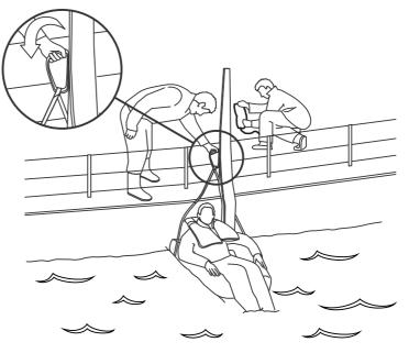
4.2.4 Once the occupant is ready, winch the module and occupant back on the board the vessel.
