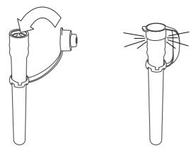
5.1.2 Rinse the recovery module with fresh water and leave to drip dry in a cool and well ventilated area.
