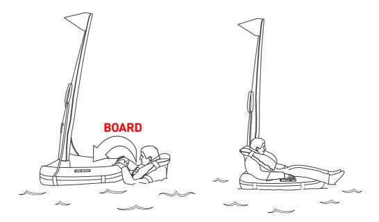
3.2.2 Ocean Safety recommend that the recovery module is approached and boarded from the front. However it is also possible to board at the side of the module.
