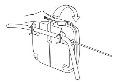
3.1.2 Upon release, the container will open and the recovery module will automatically fall outboard and automatically inflate.
