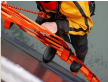
STAND OFFS, TO BRING THE LADDER AWAY FROM A FLAT SIDE
